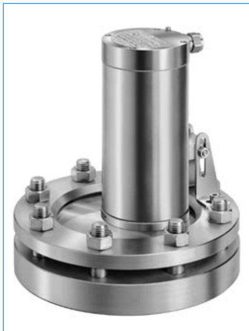
Sightglass light fitting type EdelEx 50 dH Sch K2, 50 W, 230 V, EEx d IIC T4, Ex II 2 G + D, mounted on circular sightglass to DIN 28120, PN 10, DN 150.
