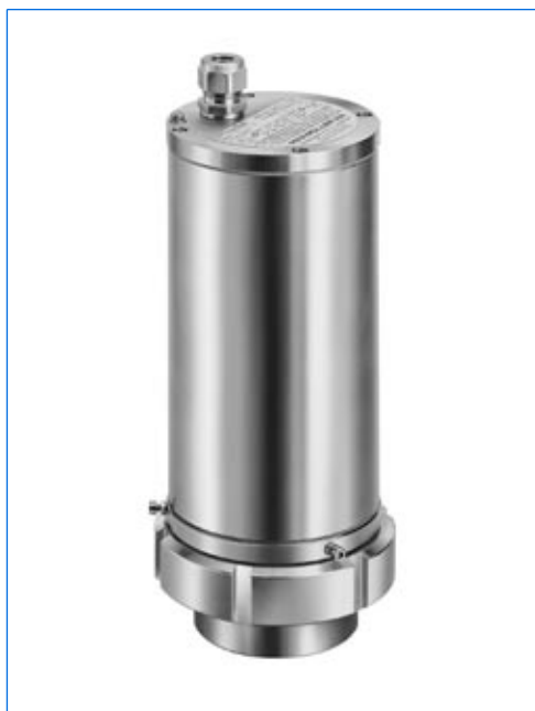
Sightglass light fitting type EdelEx G20 dH R 80 K1, 20 W, 230 V, EEx d IIC T5, Ex II 2 G + D, with intermediate flange collar fixation "R 80" mounted on a screwed sightglass similar to DIN 11851, PN 6, DN 80.
