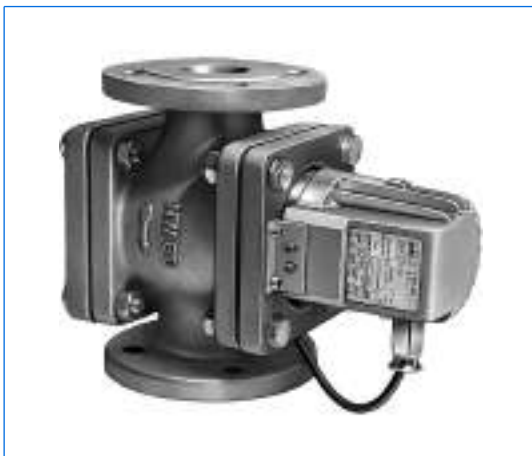
Hazardous area type FKEL 5 dH WM, Ex d IIC T6 Gb, Ex t IIC T80°C Db IP67, Ex II 2 G + D, 230 V, 5 W, with opal glass "M", on pipeline flow indicator DN 50.
