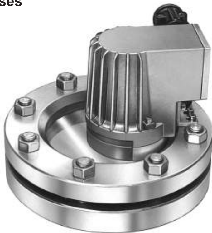
Type KEL 20 deH W, Ex d e IIC T4 Gb, Ex t IIIC T130°C Db IP67, Ex II 2 G + D, 230 V, 20 W, mounted on circular sightglass to DIN 28120, DN 125, PN 10, in 1 port version.
