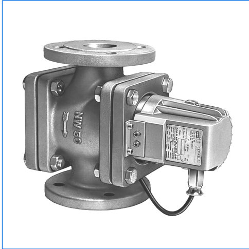
Sight flow indicator, type FDE 50, with sightglass light fitting type FKEL 5 dH WM, Ex d IIC T6 Gb, Ex t IIC T80°C Db IP67, Ex II 2 G + D, 230 V, 5 W, with opal glass screen «M»
